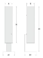
TECHNICAL FEATURES SanificaAria 30 Power supply: 230Vac ±10%, 50÷60Hz Local switch on the power cord Absorption: 24W UV-C Lamp: TC 2G11 18W Wave length UV-C: 254nm Sanitization airflow rate: 30m³/h Radiant power UV-C: 5,5W
